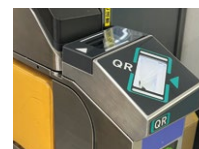
Ticket machine fitted with QR code reader and card touch payment function
