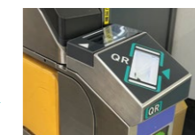
Ticket machine fitted with QR code reader and card touch payment function
